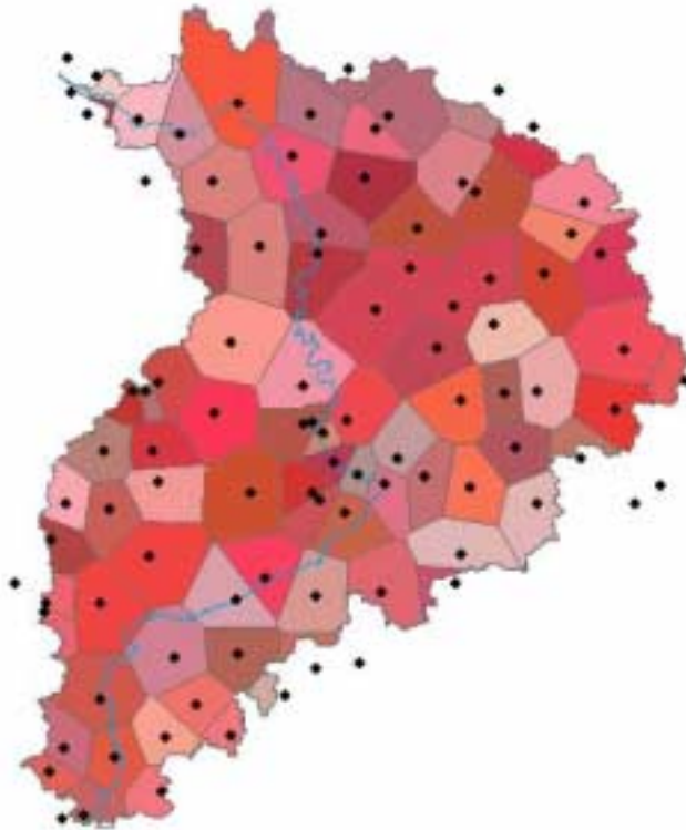
Fig. 2: 98 climate stations with daily values of radiation, precipitation, air humidity, min. and max. temperature, wind from 1989 to 2003. (Source: LfU)
